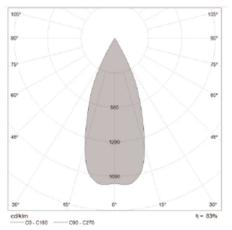
Correlated color temperature: 3000 – 6000 kelvin Rated median useful life: 50000h L70 at 25°C Luminaire input power: 15 w
